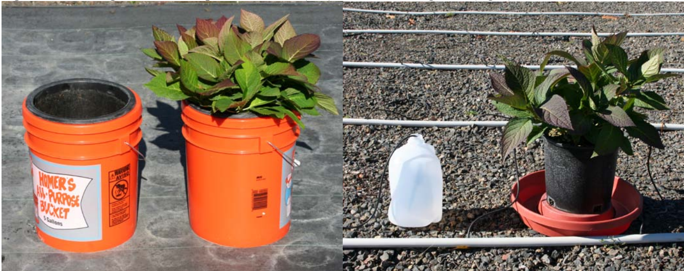
Figure 6: Leaching fraction set-up for overhead (left) and micro-irrigation (right).
