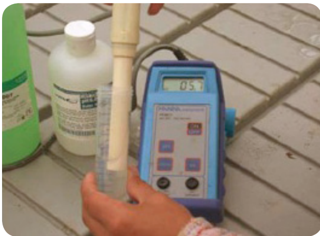
Use of EC meter to obtain reading on leachate sample.
