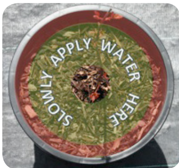
Area of the substrate surface in which water is to be applied slowly in concentric circles.
